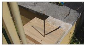
Clockwise from above. **Figure 2.** On 21 March a reference nail (perpendicular to the plane) is driven into a wooden board. A second nail is fixed next to the reference nail at an angle that produces no shadow. **Figure 3.** On 21 June at 13:00 (because of daylight saving time, solar noon is at 13:00), a third nail was driven into the same board at an angle that produces no shadow. **Figure 4.** The angle between the two nails driven on 21 March and 21 June yields the axial tilt of the Earth.
