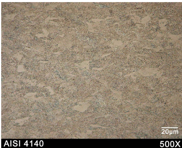
Fig. 2. Optic microstructure of AISI 4140 steel.
