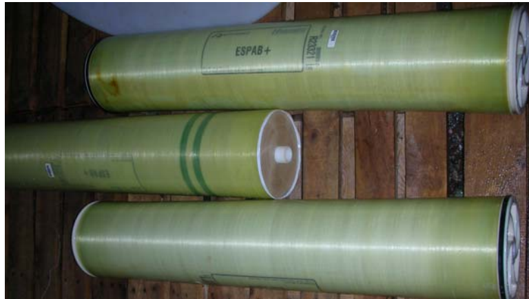
Figure 1 Hydranautics ESPAB+ membranes used in pilot RO system (see online version for colours)
