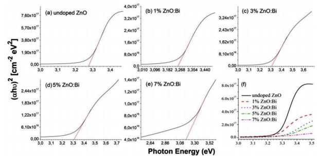
Fig. 3. Plot of  $(\alpha h\nu)^2$  versus photon energy for ZnO and ZnO:Bi thin films.
