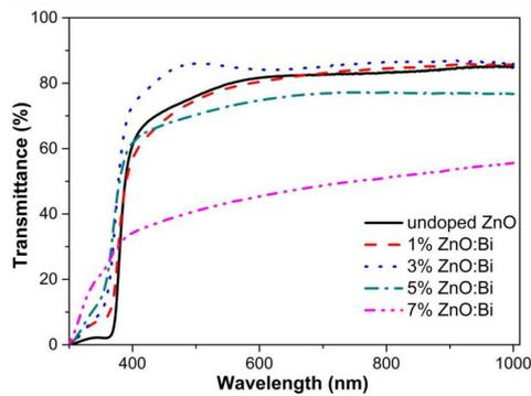
Fig. 4. Optical transmittance spectra of undoped and various Bi doped ZnO films.
