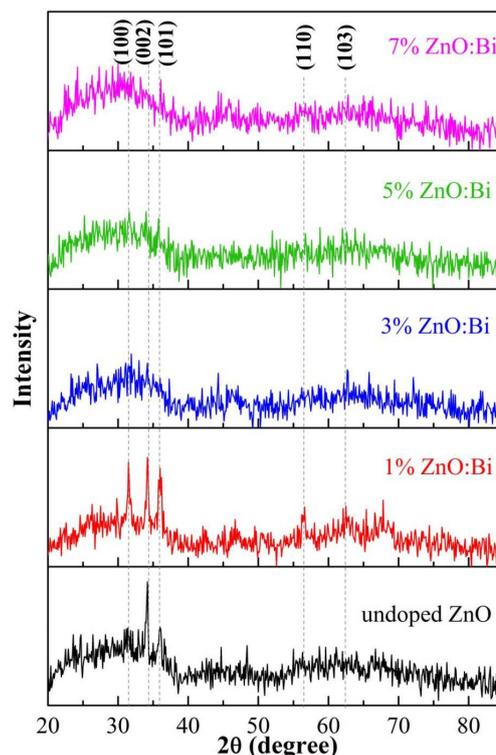
Fig. 1. X-ray diffraction spectra of the ZnO and ZnO:Bi films.
