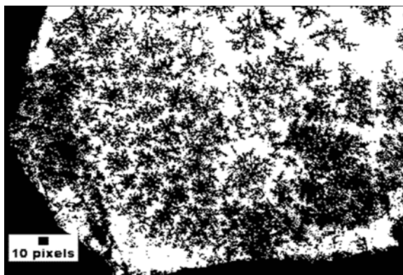
Fig. 1. Typical magnesite ore surface with MnDs. The MnDs patterns are distributed as random structure on the MO surface.
