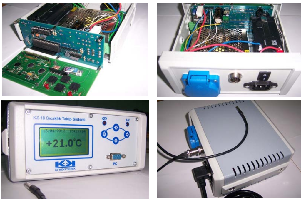
Fig.11 — Electronics card design of the developed system, layout and rear and front panels
