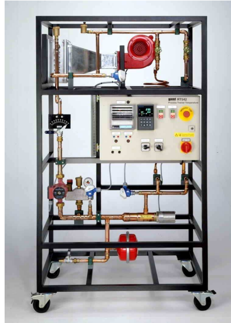
Fig. 6 Temperature Control Trainer [10]
