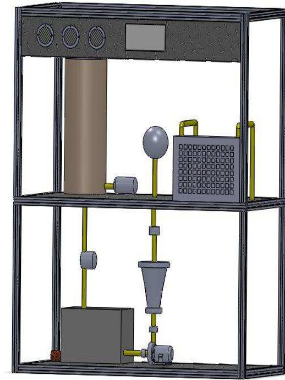
Fig. 8 Multi process control trainer
