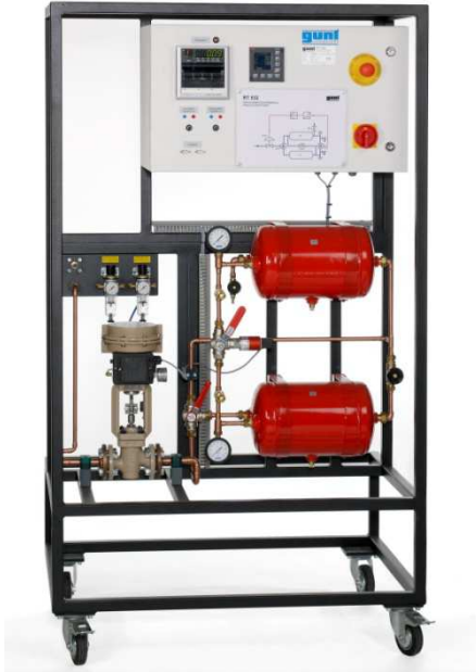
Fig. 5 Pressure Control Trainer [10]
