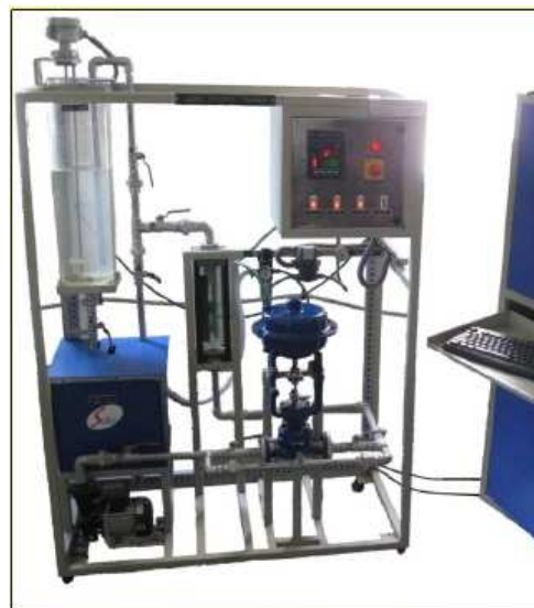
Fig. 4 Level Control Trainer [9]
