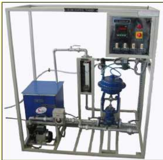
Fig. 3 Flow Control Trainer [8]
