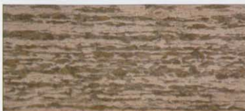
Fig. 13: Optical microscope pictures of sample 7 ( P_t=162 MPa, P_u=121.5 MPa) (500 \times )
