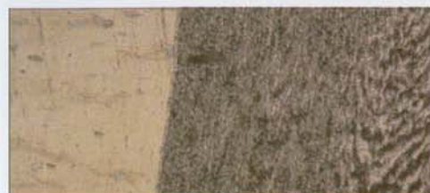
Fig. 13: Optical microscope pictures of sample 7 ( P_t=162 MPa, P_u=121.5 MPa) (500 \times )
