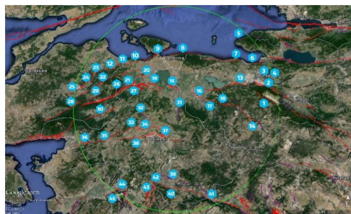
Figure 5. The active faults affecting the Susurluk (Balıkesir) settlement area (The center of the circle is the Susurluk (Balıkesir) settlement area and its diameter is 100 km. The number in parentheses is given in Table 3)
