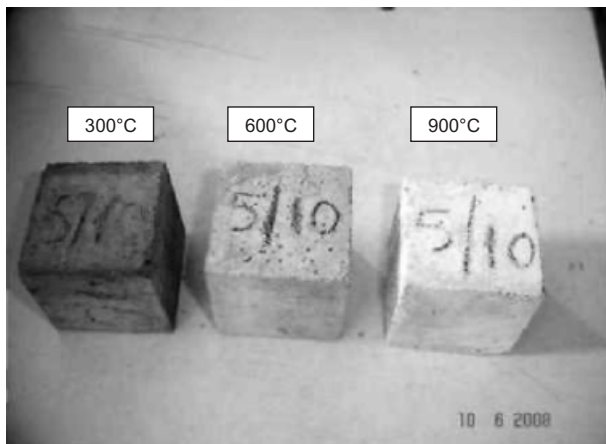
Figure 5. Exposure of the samples to elevated temperatures, 300, 600 and 900°C
