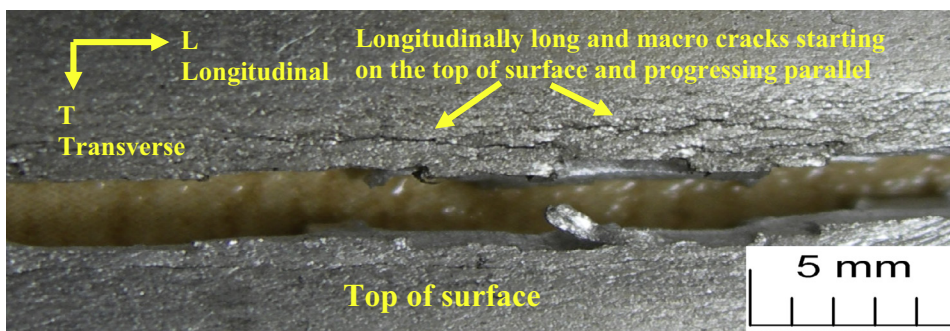
Figure 6 Macro cracks progressing on the top of the surface of the AA1100 (T) specimen.
