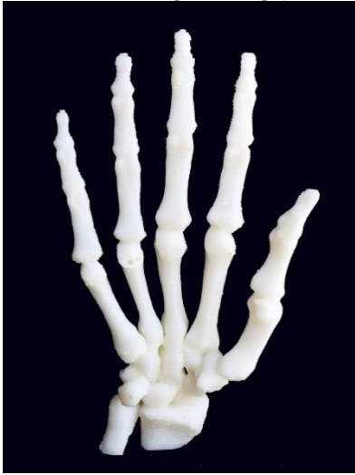
Figure 5. 3D FDM printed case study hand model
