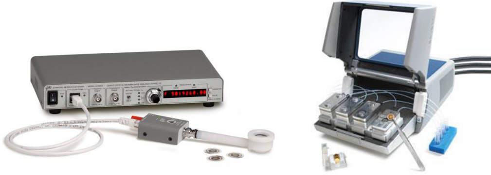
Şekil 1.4: KKM analizörleri. a) QCM200 Digital Controller (Stanford Research Systems), b) Q-Sense Analyzer (Biolin Scientific).
