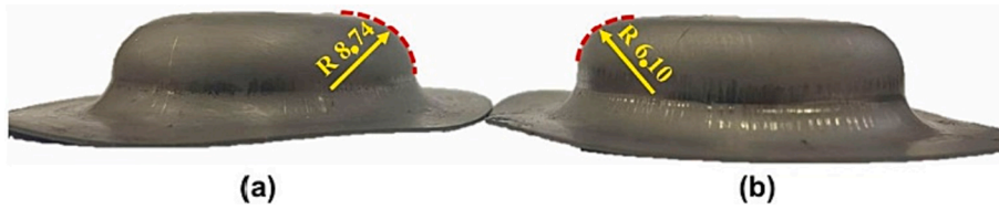
Fig. 17. The specimens formed by (a) monotonic and (b) optimized pulsating process.
