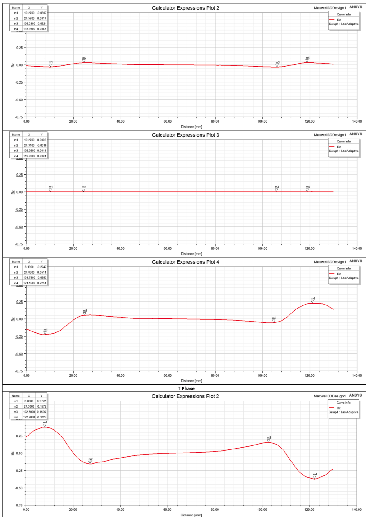
Fig. A1. Change in magnetic field magnitude along 3 polylines at the first position where the magnetic fish can rotate on the surface of the Magnetic Stirrer core (for S Phase and T Phase respectively)
