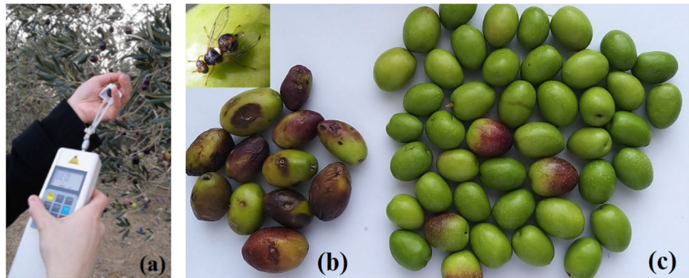
Fig. 1 a) Measurement of olive fruit removal force. b) Damaged olives c) Undamaged olives (October 20th)
