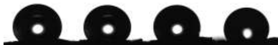
Figure 8. Sample images of water droplet CA measurements for the CSA-pumice sample (2 STs) from 141° to 117°.
