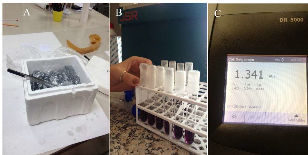
Fig. 2. Determination of proline content in liquid nitrogen after flag leaves are harvested (A), preparation of proline standards (B) and Proline readings in the spectrophotometer (C).
