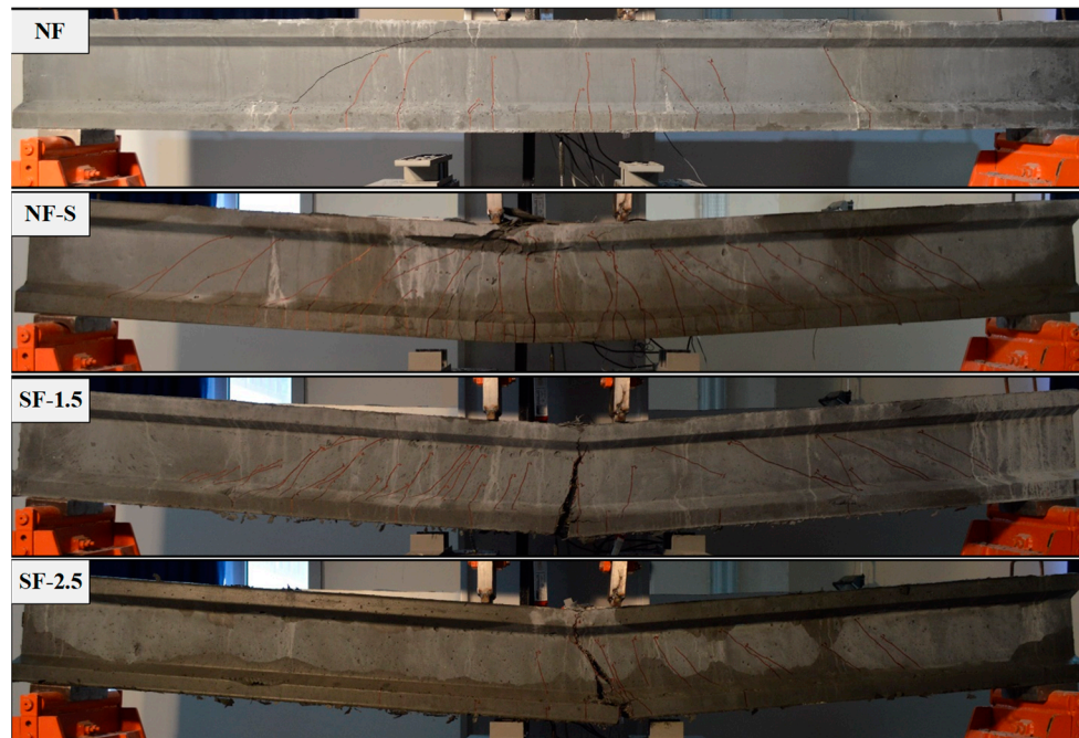
Figure 7. The failure modes of test beams.
