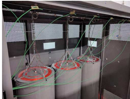
Figure 7. The view of the location of the thermocouples during measurements
