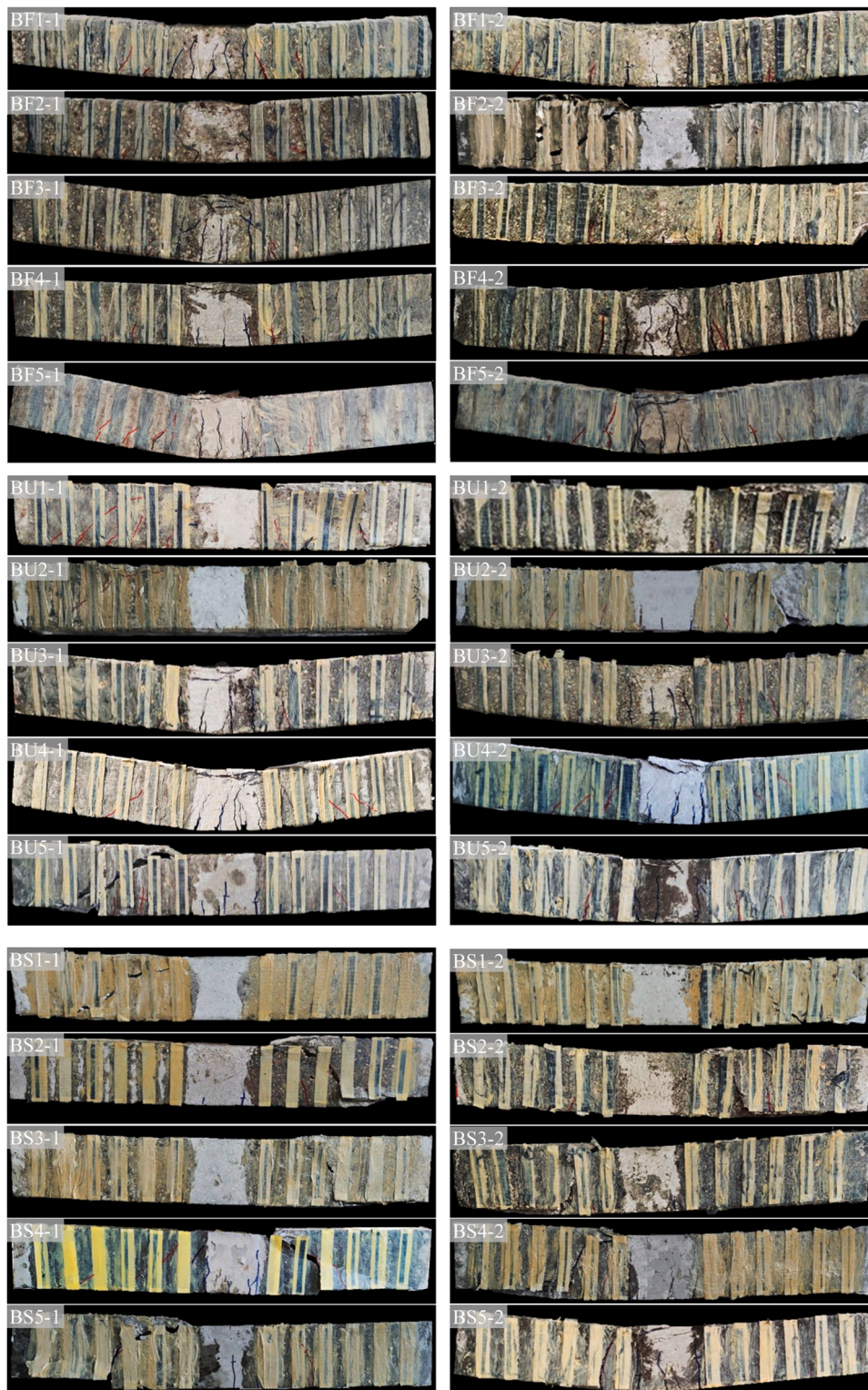
Fig. 8. Failure modes of the CFRP-strengthened beam specimens at the end of the tests.
