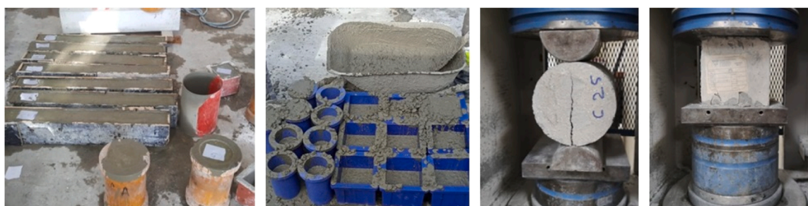
Fig. 2. Specimens prepared for compressive and splitting tests and the testing procedure.
