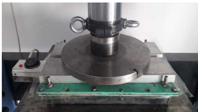
Figure 2. Composite plate manufacturing by hot-pressing.
