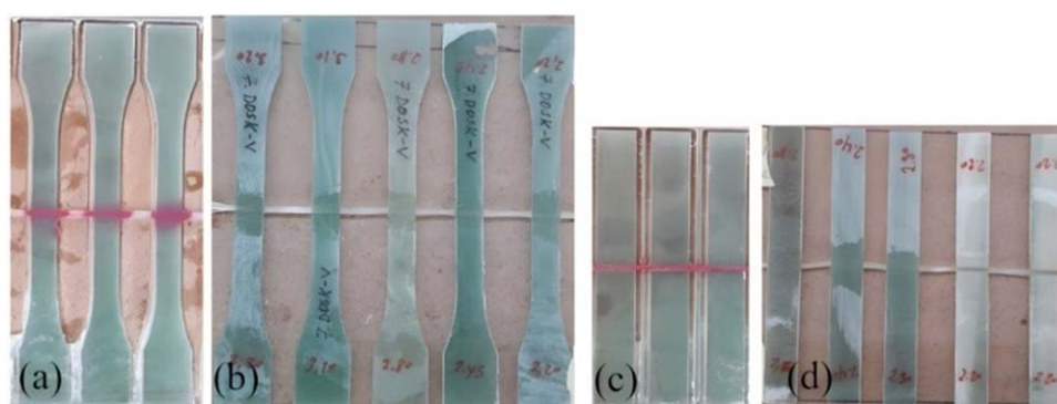
Figure 5. Tensile and flexural specimens cured at 23 °C/24 h.
