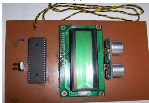
Fig.2.6: (a) Circuit diagram of distance measurement system b) photograph of distance measurement system
