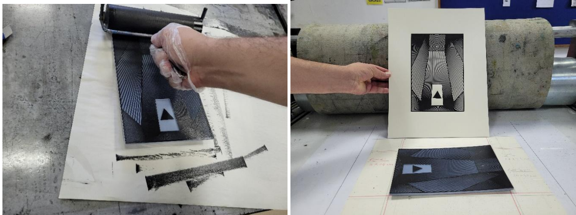
Figure 8a-b: Inking and print output from an SLA-fabricated relief matrix
