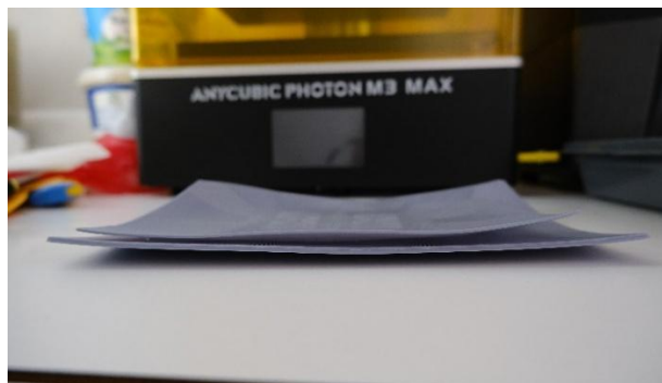
Figure 5: Thickness-dependent bending and warping behavior of SLA-printed matrices
