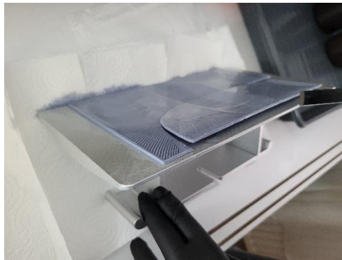
Figure 4: Fracture occurring during build plate removal of an SLA-printed relief matrix
