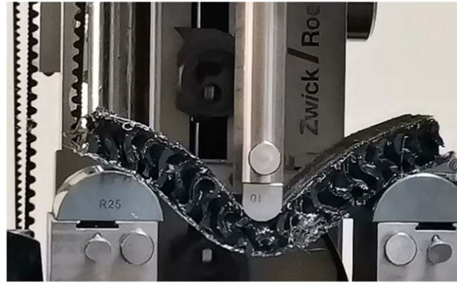
Figure 15. Three-point bending test of the composite.
