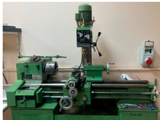
Figure 1. Emco-Maximat Mentor 10 turning-milling machine utilized in this study.
