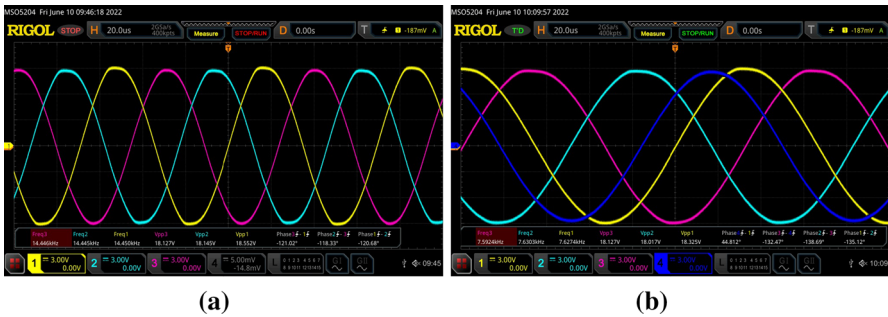
Fig. 14 Experimental output waveforms of (a) three-phase MSO, and b four-phase MSO
